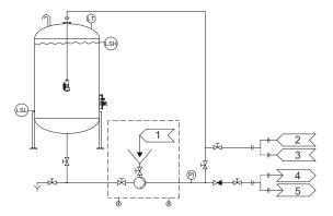
Figure 1. Example of setup with the Alfa Laval Hybrid Powder Mixer and an Alfa Laval Rotary Jet Mixer
