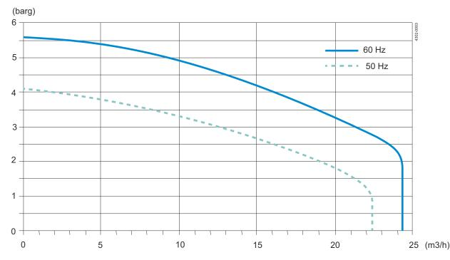
Figure 2. Pump Curve for the Alfa Laval Hybrid Powder Mixer
