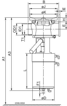
**Unique-TO connected to stub flange**
