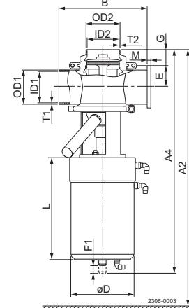
A1 + A2 = Min. clearance to allow that actuator and internal valve parts can be lifted out of the valve body. If ThinkTop is mounted, add 180 mm.
