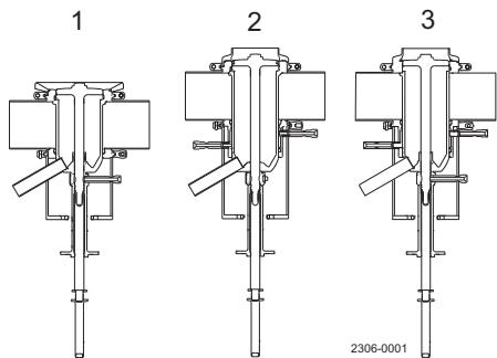
1. External CIP of leakage chamber
