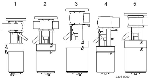
1. DN50 with tank flange, group 3 actuator including seat lift and seat push
