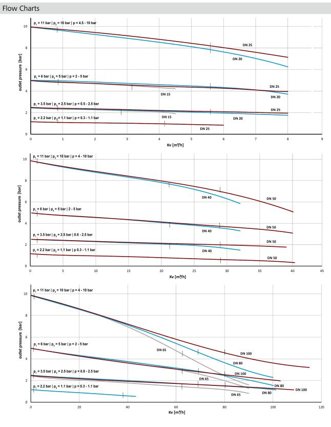
p = pressure range  $p_1 = inlet pressure$   $p_2 = adjusted outlet pressure$  = recommended working range
